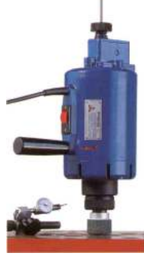
334-010 Valve seat grinder Machine is complete with self centering pilots and grinding wheels 26 - 63 mm diameter. Stone dresser included to reface grinding wheels. 220V Single phase.
