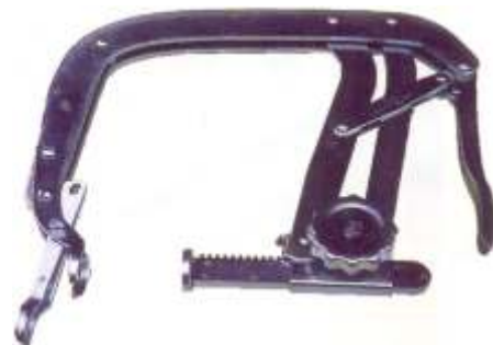
340-030 Valve spring compressor For large engines complete with two sets of jaws. Capacity 55 - 165 mm with offset jaws and 75 - 185 mm with straight jaws. Throat clearance 245 mm.
