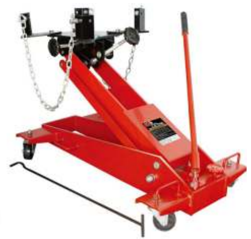
780-020 Transmission jack Trolley type 2 Ton capacity Transmission jack with adjustable cradle Minimum height 210mm Maximum height 960mm
