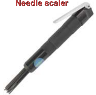
254-010 Needle scaler Ideal for removing paint, cement, rust and welding on uneven surfaces. 2800BPM. 12 Needles.
