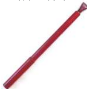
126-010 Bead knocker Suitable for truck, bus, tractor and earthmover tyres
