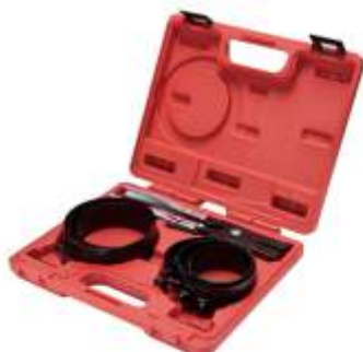
344-040 Piston ring compressor set Installs pistons from 2.7/8" to 4.3/8" (73 to 111mm). 6 Bands. Ratchet allows for bands to compress in small increments.
