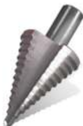
374-020 Step drill 5 to 35 mm Steps of 2 to 3mm 5, 8, 10, 12, 14, 17, 20, 22, 25, 27, 30, 32 and 35mm
