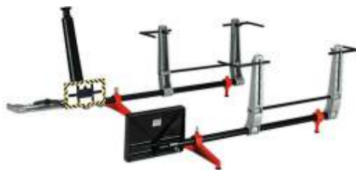
174-020 Laser toe in / out gauge (Optical type) Optical toe in / out gauge. Laser beam for accurate readings. Can be used on level floor. No need for use on lift or pit.
