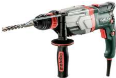
290-040 Rotary hammer drill 1100W 24mm (masonry) Variable electronic speed with forward and reverse direction. 2.8J Chiseling capacity. 1100W Power. SDS chuck but also a standard quick change keyless 13mm included. Capacity 24mm masonry.
