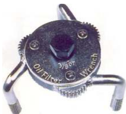
734-030 Oil filter wrench 3 Leg Loosens or tightens oil filters from 2.1/2" to 4.3/4" (60 -120 mm) diameter. Use with 3/8" square drive or 3/4" (19mm) spanner.
