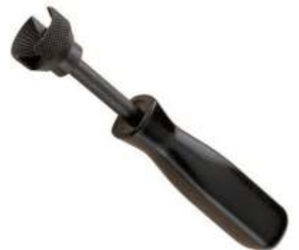
330-030 Brake spring washer tool To remove and install stubborn hold-down springs. Suitable for spring washers 5/8" to 7/8" (12 - 22mm) in diameter
