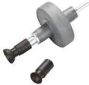
334-030 Oscillating valve lapper Unique mechanism converts rotary drill action to oscillating grinding motion. 22/28mm sucker head fits most valves.
