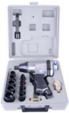
228-030 Impact wrench kit with sockets 1/2" drive Capacity 310Nm. Includes 10 impact sockets 9, 10, 11, 13, 14, 17, 19, 22, 24, 27mm, 125mm extension and an in line lubricator.
