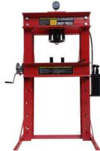
072-060 Hydraulic shop press Professional press with gauge 50 Ton Stroke 190mm Working capacity 0-800mm Includes winch to lift or lower cradle
