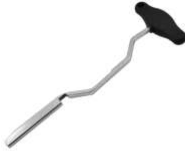
786-010 Mechatronic unit remover (DSG) Specially designed to remove load from plungers of mechatronic unit when you insert the tool between clutch lever and gear housing
