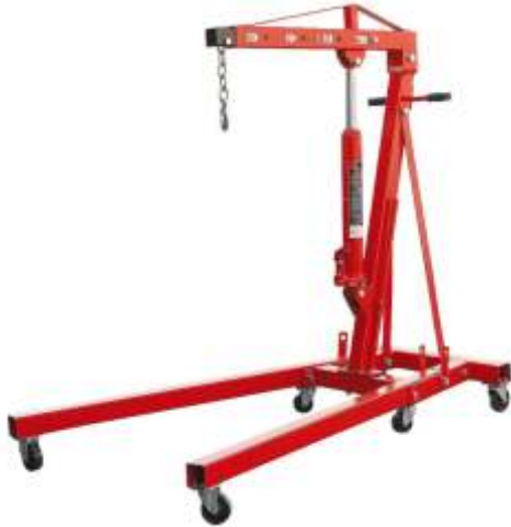
040-020 Engine crane 2 Ton capacity. Engine crane on wheels and foldable to save space when storing. Minimum height 25mm. Maximum height 2300mm.
