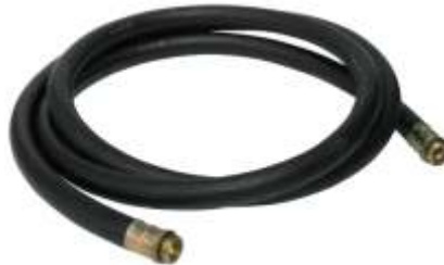
748-010 Hose with 1" fittings both sides Length 4m Maximum pressure 10Bar
