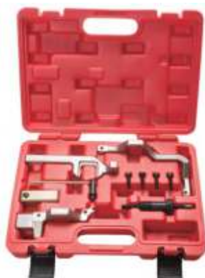
568-010 Timing tool BMW, Mini, Citroen, Peugeot N12 / N14 1.4 1.6 Petrol
