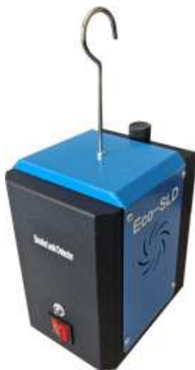
436-030 Smoke leak detector (Economy version) Produces white smoke to check intake and exhaust manifolds, valve seats and various other systems where it is difficult otherwise. Use standard baby oil to produce smoke. Complete with adaptors to connect to system.
