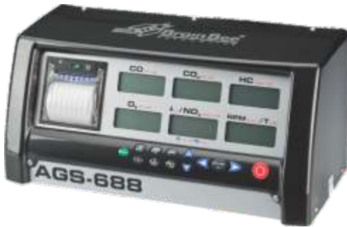
436-010 4-Gas analyser (5-Gas optional) Used to measure CO, HC, O2 and Co2 (NOX Optional) These readings can be used to analyse and adjust the most advance fuel injection and carburettor system. Lambda, AFR and corrective CO can be displayed as well. The warm up time is 3 minutes. Printer included
