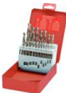
376-010 Drill set 1 to 10mm 19 Piece 1 to 10mm in each 0.5mm size
