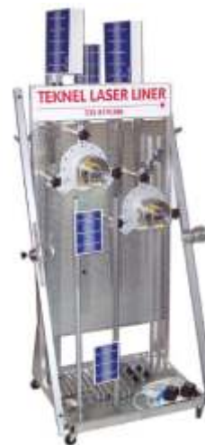
174-030 Laser wheel aligner for trucks and trailers Includes two light alloy heads to measure camber and caster. Eight targets to measure toe and thrust-line on various parts of the truck / trailer such as kingpin, draw-bar or chassis. Heavy duty set of turntables included. Wheel alignment can be done on any flat surface and takes only a few minutes to set up. Readings are accurate and reliable.
