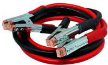
510-010 Battery booster cables (1000A) Very heavy duty cables suitable for most vehicles. Battery cables are 50m 2 and use clamps with copper tips.
