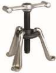
100-010 Hub puller Removes wheel hubs mounted on tapered axles. Three adjustable legs adjustable up to 190mm diameter.
