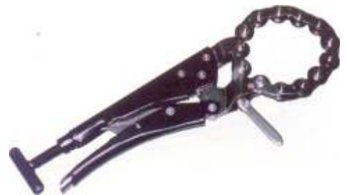
790-020 Tailpipe & tubing cutter Vice grip handle design cuts pipes easily without needing to exert pressure. Simply turn adjustment T bar in handle for further force. Can cut up to 2.5 mm thickness. Capacity 19 - 83 mm OD
