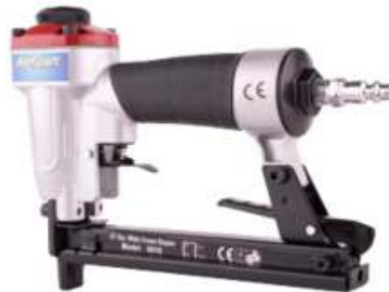
248-010 Nail gun (18 gauge (1.25mm) nails) Maximum thickness 18 gauge. Length of nails 10 to 32mm. Maximum capacity 100 nails.
