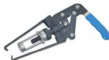
340-060 OHV Valve Spring Compressor Used on a wide range of OHV engines. Allows valve springs and valve stem oil seals to be replaced with the cylinder head mounted. Features a reversible jaw adaptor and automatic cam-action locking system to a pre-determined setting. NOT suitable for use on engines with deep seated valves.
