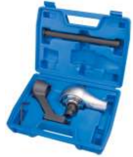
Torque multiplier By using a smaller torque wrench, much higher torques (5 times more) can be obtained Code Ratio Torque Drive 646-010 5:1 2000Nm 1/2" & 1" 646-020 5:1 2700Nm 3/4" & 1"
