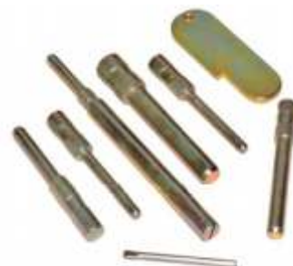
602-160 Timing tool Ford 1.6 1.8 2.5 D / TD
