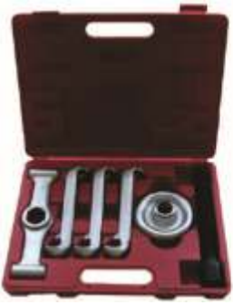
100-010 Hub puller Removes wheel hubs mounted on tapered axles. Three adjustable legs adjustable up to 190mm diameter.
