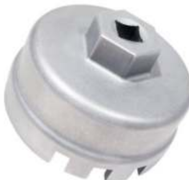
734-020 Toyota filter cup 14 Flutes x 64.5mm Steel thickness: 2.5mm Designed with 6 slots 1/2" Drive or 21mm spanner
