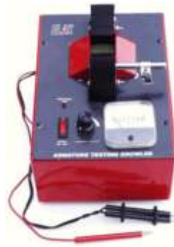
506-010 Armature growler For testing armatures on motors
