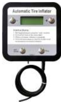
154-020 Automatic digital tyre inflator 220V Single phase. Indoor use. Inflates or deflates tyres to the selected pressure. Beeps when done. Includes wall mounting bracket.
