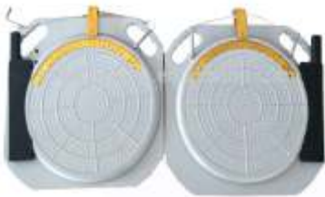
176-030 Turntable set Sold in pairs. Complete with radius gauge and rubber spacers. Full floating type 400mm x 400mm x 50mm high.
