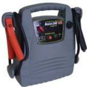
498-010 Booster pack 12V Capable of starting most petrol & diesel cars and LDV vehicles. Voltage 12V 2000A. Designed to supply high current at short intervals. Not recommended to crank problem vehicles for long durations.
