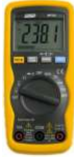
486-020 Multimeter AC & DC Voltage 0 to 1000V, AC & DC Amperage 0 to 10A (optional clamp on adaptor available to measure amperage up to 600A), frequency up to 10MHz, capacitance up to 4000µF, duty cycle , resistance up to 60MΩ, continuity tester with buzzer, auto ranging, data hold, min & max hold standard
