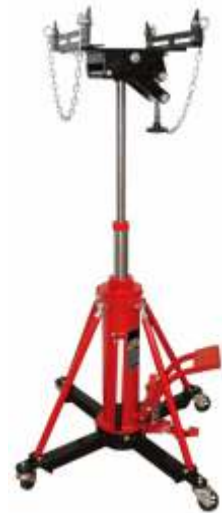
782-030 Transmission jack Pit / Lift type 1 Ton capacity Transmission jack with adjustable cradle Minimum height 855mm Maximum height 1845mm
