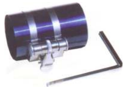
Piston ring compressors Self locking ratchet pawl allows positive locking action. Friction proof band edge makes a smooth & accurate operation. Code Height Capacity 344-010 3" 76mm 53-125mm 344-020 4" 100mm 60-175mm 344-030 6" 150mm 60-175mm
