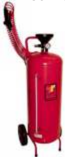
758-010 Foamer Used to apply car shampoo and detergent to vehicles. 10m hose with gun. 50L tank. Maximum pressure 8 Bar.
