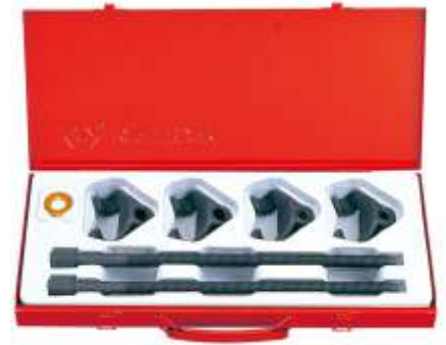
076-020 Coil spring compressor External type. Two legs with double hooks on both sides. Pressure is evenly balanced and operation is safer.
