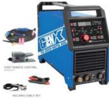
826-050 TIG / MMA welder AC / DC Suitable for aluminium welding. 5-200A. Electrode size up to 4mm. Voltage 220V. Includes earth cable, electrode cable, foot operated control and TIG torch. Optional extras, flow meter and gas. Weight 15Kg
