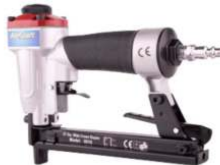
250-010 Stapler (21 gauge (0.6mm) staples) Maximum thickness 21 gauge (0.6mm). Length of staples 6 to 16mm. Maximum capacity 125 nails. Crown width 12.7mm
