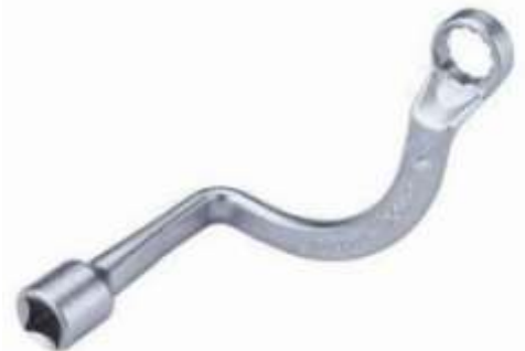
558-010 Turbo spanner 12mm Bi-hexagon spanner to be used with 3/8" Drive ratchet. To be used on VW / Audi diesel engines fitted with turbo chargers
