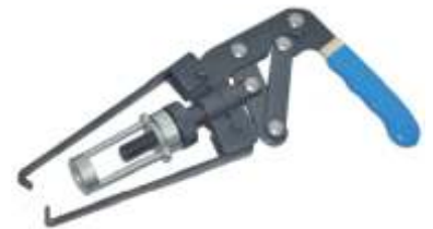
340-060 OHV Valve Spring Compressor Used on a wide range of OHV engines. Allows valve springs and valve stem oil seals to be replaced with the cylinder head mounted. Features a reversible jaw adaptor and automatic cam-action locking system to a pre-determined setting. NOT suitable for use on engines with deep seated valves.
