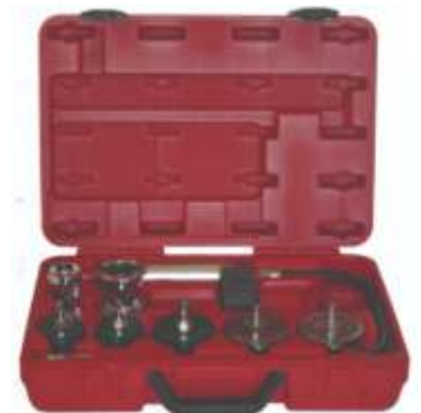
546-030 Radiator cap pressure tester Suitable for most standard radiator cap pressure testing. Pressure pump capable of testing up to 2 Bar (30 psi)
