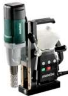
292-010 Mag base drill 1000W 32mm (Steel) Broach cutter adaptor included. 1000W Power. 16mm Geared chuck and chuck adaptor available.
