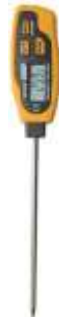
554-020 Pen type thermometer Temperature from -40 °C to 250 °C. Includes data hold, automatic power off, and minimum / maximum reading hold. Probe made of stainless steel.
