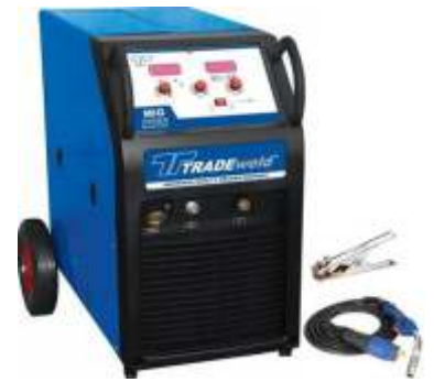
826-030 MIG welder (C02) 250A. Welding wire 0.8 to 1mm Voltage 220V. Includes cable and MIG torch. Optional extras, flow meter and gas. Weight 62Kg
