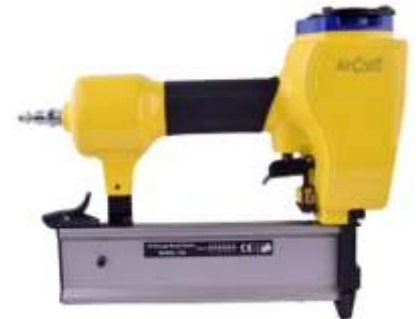
248-020 Nail gun (16 gauge (1.65mm) nails) Maximum thickness 16 gauge. Length of nails 15 to 50mm. Maximum capacity 100 nails.
