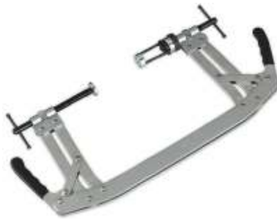
340-050 Multi valve spring compressor Suitable for use on multi-valve petrol and diesel engines with deep-seated valves. Suitable also for general use on OHC engines. Universal jaw with 55-175mm capacity and 165mm throat depth. Reversible jaw and adaptor. Twin cam action permits use from above or below valve.
