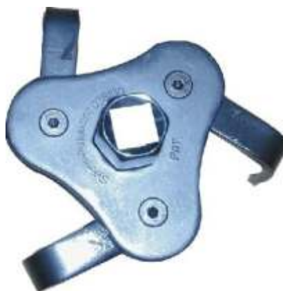
734-040 Oil filter wrench two way Removes all oil filters from 2 1/2"- 4 3/4" (65 - 120 mm). Use with 1/2" or 3/8" square drive tool.
