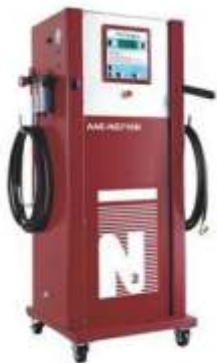
152-010 Nitrogen Generator Produces nitrogen at 42 L/min Pressure 8 Bar Suitable for truck and car wheels with built in 50L tank Complete with automatic tyre inflator / deflator
