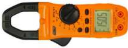
488-010 Clamp meter AC / DC Amps 0 to 800V. No need for tapping into the circuit. Simply clamp the meter over the wire. AC & DC Volts 0 to 600V, temperature, capacitance, frequency, resistance, continuity tester with buzzer and diode test. Automatic power off function.
