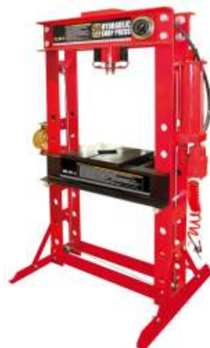
072-060 Hydraulic shop press Professional press with gauge 50 Ton Stroke 175mm Working capacity 0-890mm Includes winch to lift or lower cradle
