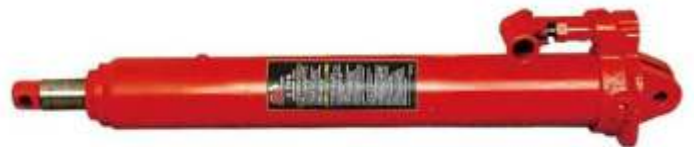
044-010 Hydraulic cylinder for engine cranes Capacity 8000 Kg. Minimum height 630mm. Maximum height 1120mm
