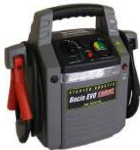
498-020 Booster pack 12V 24V Capable of starting most petrol & diesel cars, LDV's and small trucks. Voltage 12V 4000A or 24V 2000A. Designed to supply high current at short intervals. Not recommended to crank problem vehicles for long durations.
