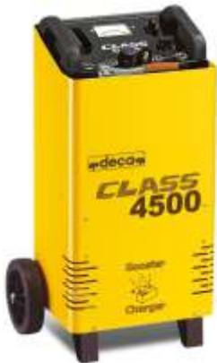
504-040 Boost battery charger on wheels 12 and 24V. Continuous charge rate of 75A. Boost charge 500A.
