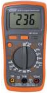
486-010 Multimeter AC / DC Voltage 0 to 500V, AC & DC Amperage 0 to 10A , transistor check (PNP or NPN), diode check, resistance up to 2MΩ, continuity tester with buzzer and data hold, min & max hold standard.
