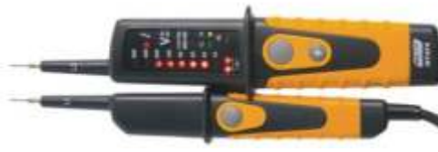
490-010 Voltage tester AC & DC Voltage 0 to 690V, phase rotation test, single pole phase check, low impedance check, polarity detection, rotary field indication and continuity test. By simply placing the probes of the tester onto the circuit under test, the meter is automatically turned on.
