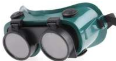
828-220 Gas welding goggles (flip front) Goggles with adjustable head strap. Can be used for grinding with dark lenses flipped up.
