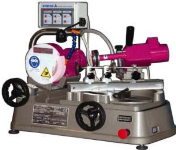
332-010 Valve refacer 230 V Single phase. Machine is complete with stone dresser. Cut valves with stem diameter from 5 - 18 mm. Special design, no need for collets to clamp valve stems.
