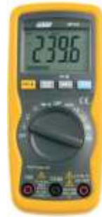
486-030 Multimeter AC & DC Voltage 0 to 1000V, AC & DC Amperage 0 to 10A (optional clamp on adaptor available to measure amperage up to 600A), frequency up to 10MHz, capacitance up to 4000µF, temperature , resistance up to 60MΩ, continuity tester with buzzer, auto ranging, data hold, min & max hold standard
