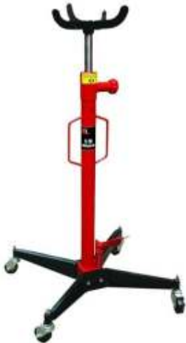
782-010 Transmission jack Pit / Lift type 500Kg capacity Transmission jack with fork Minimum height 1135mm Maximum height 1950mm
