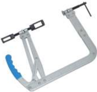
340-040 Multi valve spring compressor For multi-valve petrol & diesel engines, specially designed for difficult access & deep-seated multi-valve cylinder heads. Includes two valve spring adapters, which fit valve spring retainers up to 1" (25mm) and 1-3/16" (30mm). Jaw opening of 1-3/8" to 5-5/8" (35mm to 142mm) Throat clearance of 5-7/8" (150mm).
